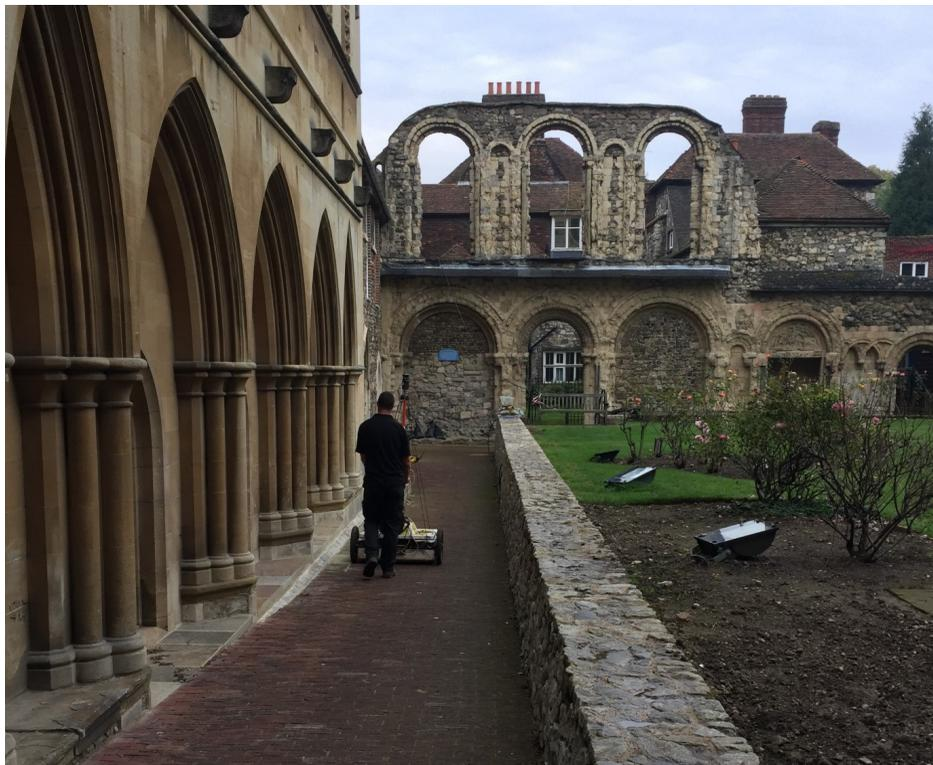
Figure 1: Richard Fleming of SUMO Stratascan surveying the north cloister walk, with the Chapter House in the background. Mounting the survey antenna on a small cart meant that the ground could be covered quickly despite the often fiddly nature of the survey area.
